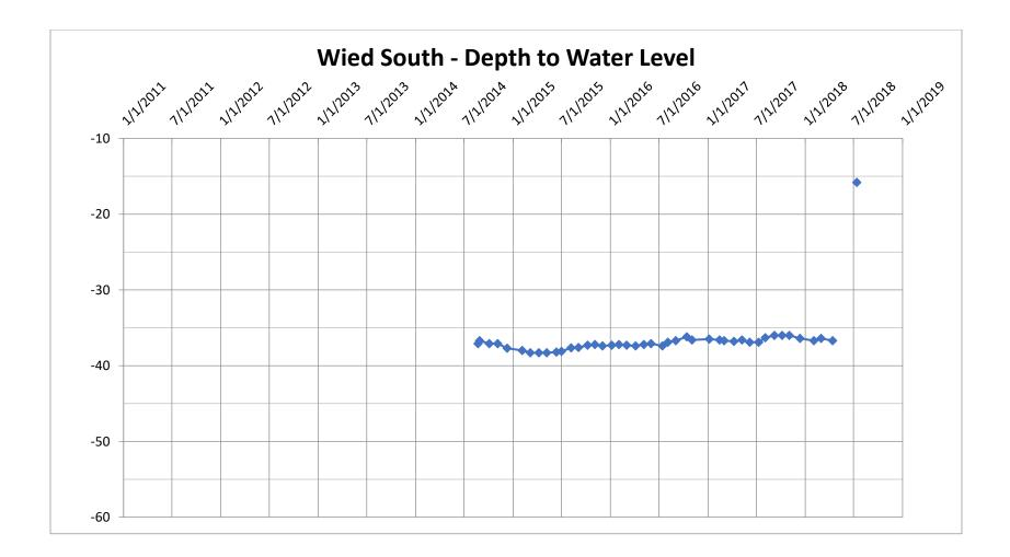
Well Designation: Wied S; State Well #: NA; Well Depth: 90'; Drill Date: NA; Screen Interval: NA'
